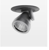
Semi-recessed luminaire with LED, rated life of the LED L80/B10 > 50000 h, colour rendering index CRI > 90, chromaticity tolerance 2 SDCM (initial), reflector with circular light distribution pattern, reflector pure aluminium 99,99% in MIRO-Silver®, segmented and faceted, 3D lens silicon to reduce the proportion of scattered light, die-cast aluminium, powder-coated, rotation angle 400°, swivel angle +85° / -85°, stratosilver, separate driver unit
