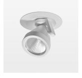
Semi-recessed luminaire with LED, rated life of the LED L80/B10 > 50000 h, colour rendering index CRI > 96, chromaticity tolerance 2 SDCM (initial), reflector with circular light distribution pattern, reflector pure aluminium 99,99% in MIRO-Silver®, segmented and faceted, 3D lens silicon to reduce the proportion of scattered light, die-cast aluminium, powder-coated, rotation angle 400°, swivel angle +85° / -85°, stratowhite, separate driver unit
