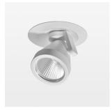
Semi-recessed luminaire with LED, rated life of the LED L80/B10 > 50000 h, colour rendering index CRI > 96, chromaticity tolerance 2 SDCM (initial), reflector with circular light distribution pattern, reflector pure aluminium 99,99% in MIRO-Silver®, segmented and faceted, 3D lens silicon to reduce the proportion of scattered light, die-cast aluminium, powder-coated, rotation angle 400°, swivel angle +85° / -85°, stratowhite, separate driver unit
