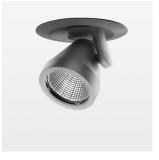
Semi-recessed luminaire with LED, rated life of the LED L80/B10 > 50000 h, colour rendering index CRI > 90, chromaticity tolerance 2 SDCM (initial), reflector with circular light distribution pattern, reflector pure aluminium 99,99% in MIRO-Silver®, segmented and faceted, 3D lens silicon to reduce the proportion of scattered light, die-cast aluminium, powder-coated, rotation angle 400°, swivel angle +85°/-85°, stratosilver, potentiometer to adjust the brightness, separate driver unit
