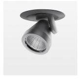
Semi-recessed luminaire with LED, rated life of the LED L80/B10 > 50000 h, colour rendering index CRI > 96, chromaticity tolerance 2 SDCM (initial), reflector with circular light distribution pattern, reflector pure aluminium 99,99% in MIRO-Silver®, segmented and faceted, 3D lens silicon to reduce the proportion of scattered light, die-cast aluminium, powder-coated, rotation angle 400°, swivel angle +85°/-85°, stratosilver, potentiometer to adjust the brightness, separate driver unit
