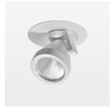
Semi-recessed luminaire with LED, rated life of the LED L80/B10 > 50000 h, colour rendering index CRI > 90, chromaticity tolerance 2 SDCM (initial), reflector with circular light distribution pattern, reflector pure aluminium 99,99% in MIRO-Silver®, segmented and faceted, 3D lens silicon to reduce the proportion of scattered light, die-cast aluminium, powder-coated, rotation angle 400°, swivel angle +85°/-85°, stratowhite, potentiometer to adjust the brightness, separate driver unit
