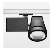
Surface-mounted luminaire with LED, rated life of the LED L80/B10 > 50000 h, chromaticity tolerance 2 SDCM (initial), reflector with oval light distribution pattern, reflector pure aluminium 99,99% in MIRO-Silver®, rotation angle 350°, swivel angle 210°, luminaire housing die-cast aluminium, powder-coated, stratoblack
