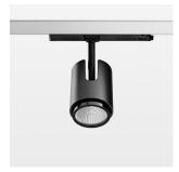
Surface-mounted luminaire with LED, rated life of the LED L80/B10 > 50000 h, chromaticity tolerance 2 SDCM (initial), , reflector with circular light distribution pattern, reflector pure aluminium 99,99% in MIRO-Silver®, segmented and faceted, exchangeable reflector unit in high-sheen black plastic, with glass cover, luminaire head die-cast aluminium, powder-coated, rotation angle 330°, swivel angle +/-90°, luminaire head/retention arm die-cast aluminium, stratoblack
