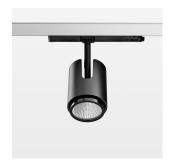
Surface-mounted luminaire with LED, rated life of the LED L80/B10 > 50000 h, chromaticity tolerance 3 SDCM (initial), , reflector with circular light distribution pattern, reflector pure aluminium 99,99% in MIRO-Silver®, segmented and faceted, exchangeable reflector unit in high-sheen black plastic, with glass cover, luminaire head die-cast aluminium, powder-coated, rotation angle 330°, swivel angle +/-90°, luminaire head/retention arm die-cast aluminium, stratoblack
