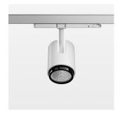
Surface-mounted luminaire with LED, rated life of the LED L80/B10 > 50000 h, chromaticity tolerance 2 SDCM (initial), , reflector with circular light distribution pattern, reflector pure aluminium 99,99% in MIRO-Silver®, segmented and faceted, exchangeable reflector unit in high-sheen black plastic, with glass cover, luminaire head die-cast aluminium, powder-coated, rotation angle 330°, swivel angle +/-90°, luminaire head/retention arm die-cast aluminium, stratowhite
