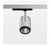
Surface-mounted luminaire with LED, rated life of the LED L80/B10 > 50000 h, chromaticity tolerance 2 SDCM (initial), , reflector with circular light distribution pattern, reflector pure aluminium 99,99% in MIRO-Silver®, segmented and faceted, exchangeable reflector unit in high-sheen black plastic, with glass cover, luminaire head die-cast aluminium, powder-coated, rotation angle 330°, swivel angle +/-90°, luminaire head/retention arm die-cast aluminium, stratosilver
