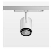
Surface-mounted luminaire with LED, rated life of the LED L80/B10 > 50000 h, chromaticity tolerance 3 SDCM (initial), , reflector with circular light distribution pattern, reflector pure aluminium 99,99% in MIRO-Silver®, segmented and faceted, exchangeable reflector unit in high-sheen black plastic, with glass cover, luminaire head die-cast aluminium, powder-coated, rotation angle 330°, swivel angle +/-90°, luminaire head/retention arm die-cast aluminium, stratowhite
