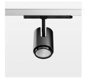
Surface-mounted luminaire with LED, rated life of the LED L80/B10 > 50000 h, chromaticity tolerance 2 SDCM (initial), , reflector with circular light distribution pattern, reflector pure aluminium 99,99% in MIRO-Silver®, segmented and faceted, exchangeable reflector unit in high-sheen black plastic, with glass cover, luminaire head die-cast aluminium, powder-coated, rotation angle 330°, swivel angle +90°/-90°, luminaire head/retention arm die-cast aluminium, stratoblack
