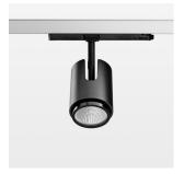
Surface-mounted luminaire with LED, rated life of the LED L80/B10 > 50000 h, chromaticity tolerance 3 SDCM (initial), , reflector with circular light distribution pattern, reflector pure aluminium 99,99% in MIRO-Silver®, segmented and faceted, exchangeable reflector unit in high-sheen black plastic, with glass cover, luminaire head die-cast aluminium, powder-coated, rotation angle 330°, swivel angle +90°/-90°, luminaire head/retention arm die-cast aluminium, stratoblack
