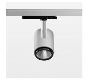
Surface-mounted luminaire with LED, rated life of the LED L80/B10 > 50000 h, chromaticity tolerance 3 SDCM (initial), , reflector with circular light distribution pattern, reflector pure aluminium 99,99% in MIRO-Silver®, segmented and faceted, exchangeable reflector unit in high-sheen black plastic, with glass cover, luminaire head die-cast aluminium, powder-coated, rotation angle 330°, swivel angle +90°/-90°, luminaire head/retention arm die-cast aluminium, stratosilver
