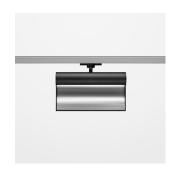
Surface-mounted wallwasher with LED, rated life of the LED L80/B10 > 50000 h, colour rendering index CRI > 90, chromaticity tolerance 3 SDCM (initial), reflector with asymmetrical light distribution pattern, reflector pure aluminium 99,99% in MIRO-Silver®, end caps die-cast aluminium, powder-coated, rotation angle 330°, luminaire housing aluminium extrusion profile, stratoblack
