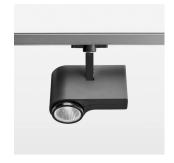
Surface-mounted luminaire with LED, rated life of the LED L80/B10 > 50000 h, colour rendering index CRI > 80, chromaticity tolerance 2 SDCM (initial), reflector with circular light distribution pattern, reflector pure aluminium 99,99% in MIRO-Silver®, segmented and faceted, exchangeable reflector unit in high-sheen black plastic, with glass cover, rotation angle 330°, swivel angle 90°, luminaire housing die-cast aluminium, powder-coated, stratoblack
