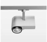
Surface-mounted luminaire with LED, rated life of the LED L80/B10 > 50000 h, colour rendering index CRI > 96, chromaticity tolerance 2 SDCM (initial), reflector with circular light distribution pattern, reflector pure aluminium 99,99% in MIRO-Silver®, segmented and faceted, exchangeable reflector unit in high-sheen black plastic, with glass cover, rotation angle 330°, swivel angle 90°, luminaire housing die-cast aluminium, powder-coated, stratosilver
