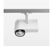
Surface-mounted luminaire with LED, rated life of the LED L80/B10 > 50000 h, chromaticity tolerance 3 SDCM (initial), reflector with circular light distribution pattern, reflector pure aluminium 99,99% in MIRO-Silver®, segmented and faceted, exchangeable reflector unit in high-sheen black plastic, with glass cover, rotation angle 330°, swivel angle 90°, luminaire housing diecast aluminium, powder-coated, stratowhite
