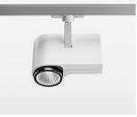
Surface-mounted luminaire with LED, rated life of the LED L80/B10 > 50000 h, colour rendering index CRI > 96, chromaticity tolerance 3 SDCM (initial), reflector with circular light distribution pattern, reflector pure aluminium 99,99% in MIRO-Silver®, segmented and faceted, exchangeable reflector unit in high-sheen black plastic, with glass cover, rotation angle 330°, swivel angle 90°, luminaire housing die-cast aluminium, powder-coated, stratowhite
