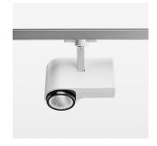
Surface-mounted luminaire with LED, rated life of the LED L80/B10 > 50000 h, chromaticity tolerance 2 SDCM (initial), reflector with circular light distribution pattern, reflector pure aluminium 99,99% in MIRO-Silver®, segmented and faceted, exchangeable reflector unit in high-sheen black plastic, with glass cover, rotation angle 330°, swivel angle 90°, luminaire housing diecast aluminium, powder-coated, stratowhite
