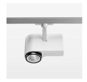
Surface-mounted luminaire with LED, rated life of the LED L80/B10 > 50000 h, chromaticity tolerance 3 SDCM (initial), reflector with circular light distribution pattern, reflector pure aluminium 99,99% in MIRO-Silver®, segmented and faceted, exchangeable reflector unit in high-sheen black plastic, with glass cover, rotation angle 330°, swivel angle 90°, luminaire housing diecast aluminium, powder-coated, stratowhite
