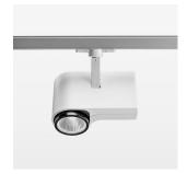
Surface-mounted luminaire with LED, rated life of the LED L80/B10 > 50000 h, colour rendering index CRI > 96, chromaticity tolerance 3 SDCM (initial), reflector with circular light distribution pattern, reflector pure aluminium 99,99% in MIRO-Silver®, segmented and faceted, exchangeable reflector unit in high-sheen black plastic, with glass cover, rotation angle 330°, swivel angle 90°, luminaire housing die-cast aluminium, powder-coated, stratowhite
