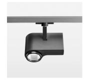
Surface-mounted luminaire with LED, rated life of the LED L80/B10 > 50000 h, chromaticity tolerance 3 SDCM (initial), LED hybrid technology, 3D silicone lens to reduce the proportion of scattered light, reflector with oval light distribution pattern, reflector pure aluminium 99,99% in MIRO-Silver®, segmented, exchangeable reflector unit in high-sheen black plastic, with glass cover, rotation angle 330°, swivel angle 90°, luminaire housing die-cast aluminium, powder-coated, stratoblack
