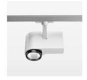
Surface-mounted luminaire with LED, rated life of the LED L80/B10 > 50000 h, chromaticity tolerance 3 SDCM (initial), LED hybrid technology, 3D silicone lens to reduce the proportion of scattered light, reflector with oval light distribution pattern, reflector pure aluminium 99,99% in MIRO-Silver®, segmented, exchangeable reflector unit in high-sheen black plastic, with glass cover, rotation angle 330°, swivel angle 90°, luminaire housing die-cast aluminium, powder-coated, stratowhite
