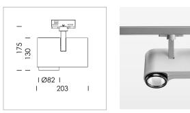
Surface-mounted luminaire with LED, rated life of the LED L80/B10 > 50000 h, chromaticity tolerance 3 SDCM (initial), LED hybrid technology, 3D silicone lens to reduce the proportion of scattered light, reflector with oval light distribution pattern, reflector pure aluminium 99,99% in MIRO-Silver®, segmented, exchangeable reflector unit in high-sheen black plastic, with glass cover, rotation angle 330°, swivel angle 90°, luminaire housing die-cast aluminium, powder-coated, stratosilver
