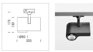
Surface-mounted luminaire with LED, rated life of the LED L80/B10 > 50000 h, chromaticity tolerance 2 SDCM (initial), LED hybrid technology, 3D silicone lens to reduce the proportion of scattered light, reflector with oval light distribution pattern, reflector pure aluminium 99,99% in MIRO-Silver®, segmented, exchangeable reflector unit in high-sheen black plastic, with glass cover, rotation angle 330°, swivel angle 90°, luminaire housing die-cast aluminium, powder-coated, stratoblack
