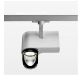
Surface-mounted luminaire with LED, rated life of the LED L80/B10 > 50000 h, chromaticity tolerance 2 SDCM (initial), reflector with asymmetrical light distribution pattern, primary reflector and kick reflector 99% pure aluminium in MIRO-Silver®, attachment with kick reflector to the ceiling approach of the light cone, exchangeable reflector unit in high-sheen black plastic, with glass cover, rotation angle 330°, swivel angle 90°, luminaire housing die-cast aluminium, powder-coated, stratosilver
