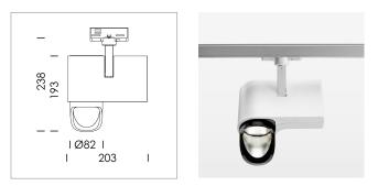
Surface-mounted luminaire with LED, rated life of the LED L80/B10 > 50000 h, chromaticity tolerance 2 SDCM (initial), reflector with asymmetrical light distribution pattern, primary reflector and kick reflector 99% pure aluminium in MIRO-Silver®, attachment with kick reflector to the ceiling approach of the light cone, exchangeable reflector unit in high-sheen black plastic, with glass cover, rotation angle 330°, swivel angle 90°, luminaire housing die-cast aluminium, powder-coated, stratowhite
