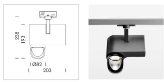
Surface-mounted luminaire with LED, rated life of the LED L80/B10 > 50000 h, chromaticity tolerance 3 SDCM (initial), reflector with asymmetrical light distribution pattern, primary reflector and kick reflector 99% pure aluminium in MIRO-Silver®, attachment with kick reflector to the ceiling approach of the light cone, exchangeable reflector unit in high-sheen black plastic, with glass cover, rotation angle 330°, swivel angle 90°, luminaire housing die-cast aluminium, powder-coated, stratoblack
