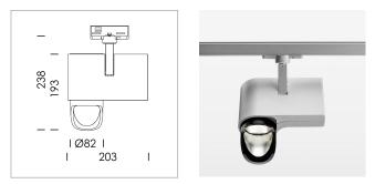
Surface-mounted luminaire with LED, rated life of the LED L80/B10 > 50000 h, chromaticity tolerance 2 SDCM (initial), reflector with asymmetrical light distribution pattern, primary reflector and kick reflector 99% pure aluminium in MIRO-Silver®, attachment with kick reflector to the ceiling approach of the light cone, exchangeable reflector unit in high-sheen black plastic, with glass cover, rotation angle 330°, swivel angle 90°, luminaire housing die-cast aluminium, powder-coated, stratosilver
