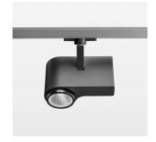
Surface-mounted luminaire with LED, rated life of the LED L80/B10 > 50000 h, colour rendering index CRI > 90, chromaticity tolerance 2 SDCM (initial), reflector with circular light distribution pattern, reflector pure aluminium 99,99% in MIRO-Silver®, segmented and faceted, exchangeable reflector unit in high-sheen black plastic, with glass cover, rotation angle 330°, swivel angle 90°, luminaire housing die-cast aluminium, powder-coated, stratoblack
