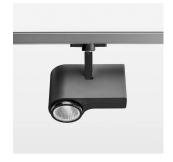
Surface-mounted luminaire with LED, rated life of the LED L80/B10 > 50000 h, chromaticity tolerance 2 SDCM (initial), , reflector with circular light distribution pattern, reflector pure aluminium 99,99% in MIRO-Silver®, segmented and faceted, exchangeable reflector unit in high-sheen black plastic, with glass cover, rotation angle 330°, swivel angle 90°, luminaire housing diecast aluminium, powder-coated, stratoblack
