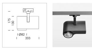
Surface-mounted luminaire with LED, rated life of the LED L80/B10 > 50000 h, chromaticity tolerance 3 SDCM (initial), , reflector with circular light distribution pattern, reflector pure aluminium 99,99% in MIRO-Silver®, segmented and faceted, exchangeable reflector unit in high-sheen black plastic, with glass cover, rotation angle 330°, swivel angle 90°, luminaire housing diecast aluminium, powder-coated, stratoblack
