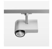
Surface-mounted luminaire with LED, rated life of the LED L80/B10 > 50000 h, colour rendering index CRI > 90, chromaticity tolerance 2 SDCM (initial), reflector with circular light distribution pattern, reflector pure aluminium 99,99% in MIRO-Silver®, segmented and faceted, exchangeable reflector unit in high-sheen black plastic, with glass cover, rotation angle 330°, swivel angle 90°, luminaire housing die-cast aluminium, powder-coated, stratosilver
