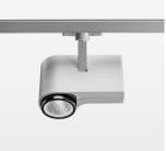
Surface-mounted luminaire with LED, rated life of the LED L80/B10 > 50000 h, chromaticity tolerance 2 SDCM (initial), , reflector with circular light distribution pattern, reflector pure aluminium 99,99% in MIRO-Silver®, segmented and faceted, exchangeable reflector unit in high-sheen black plastic, with glass cover, rotation angle 330°, swivel angle 90°, luminaire housing diecast aluminium, powder-coated, stratosilver
