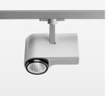
Surface-mounted luminaire with LED, rated life of the LED L80/B10 > 50000 h, colour rendering index CRI > 90, chromaticity tolerance 2 SDCM (initial), , reflector with circular light distribution pattern, reflector pure aluminium 99,99% in MIRO-Silver®, segmented and faceted, exchangeable reflector unit in high-sheen black plastic, with glass cover, rotation angle 330°, swivel angle 90°, luminaire housing die-cast aluminium, powder-coated, stratosilver
