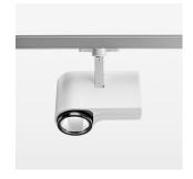
Surface-mounted luminaire with LED, rated life of the LED L80/B10 > 50000 h, chromaticity tolerance 3 SDCM (initial), LED hybrid technology, 3D silicone lens to reduce the proportion of scattered light, reflector with oval light distribution pattern, reflector pure aluminium 99,99% in MIRO-Silver®, segmented, exchangeable reflector unit in high-sheen black plastic, with glass cover, rotation angle 330°, swivel angle 90°, luminaire housing die-cast aluminium, powder-coated, stratowhite
