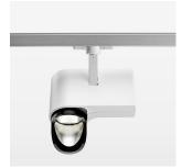
Surface-mounted luminaire with LED, rated life of the LED L80/B10 > 50000 h, chromaticity tolerance 3 SDCM (initial), reflector with asymmetrical light distribution pattern, primary reflector and kick reflector 99% pure aluminium in MIRO-Silver®, attachment with kick reflector to the ceiling approach of the light cone, exchangeable reflector unit in high-sheen black plastic, with glass cover, rotation angle 330°, swivel angle 90°, luminaire housing die-cast aluminium, powder-coated, stratowhite
