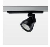
Surface-mounted luminaire with LED, rated life of the LED L80/B10 > 50000 h, colour rendering index CRI > 96, chromaticity tolerance 2 SDCM (initial), reflector with circular light distribution pattern, reflector pure aluminium 99,99% in MIRO-Silver®, rotation angle 330°, swivel angle +85°/-85°, luminaire head/retention arm die-cast aluminium, powder-coated, stratoblack
