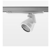
Surface-mounted luminaire with LED, rated life of the LED L80/B10 > 50000 h, colour rendering index CRI > 96, chromaticity tolerance 3 SDCM (initial), reflector with circular light distribution pattern, reflector pure aluminium 99,99% in MIRO-Silver®, rotation angle 330°, swivel angle +85°/-85°, luminaire head/retention arm die-cast aluminium, powder-coated, stratowhite
