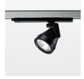
Surface-mounted luminaire with LED, rated life of the LED L80/B10 > 50000 h, colour rendering index CRI > 96, chromaticity tolerance 2 SDCM (initial), reflector with oval light distribution pattern, reflector pure aluminium 99,99% in MIRO-Silver®, rotation angle 330°, swivel angle +85°/-85°, luminaire head/retention arm die-cast aluminium, powder-coated, stratoblack
