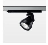
Surface-mounted luminaire with LED, rated life of the LED L80/B10 > 50000 h, colour rendering index CRI > 96, chromaticity tolerance 3 SDCM (initial), reflector with oval light distribution pattern, reflector pure aluminium 99,99% in MIRO-Silver®, rotation angle 330°, swivel angle +85°/-85°, luminaire head/retention arm die-cast aluminium, powder-coated, stratoblack
