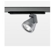
Surface-mounted luminaire with LED, rated life of the LED L80/B10 > 50000 h, colour rendering index CRI > 96, chromaticity tolerance 2 SDCM (initial), reflector with oval light distribution pattern, reflector pure aluminium 99,99% in MIRO-Silver®, rotation angle 330°, swivel angle +85°/-85°, luminaire head/retention arm die-cast aluminium, powder-coated, stratosilver
