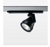
Surface-mounted luminaire with LED, rated life of the LED L80/B10 > 50000 h, colour rendering index CRI > 96, chromaticity tolerance 3 SDCM (initial), reflector with oval light distribution pattern, reflector pure aluminium 99,99% in MIRO-Silver®, rotation angle 330°, swivel angle +85°/-85°, luminaire head/retention arm die-cast aluminium, powder-coated, stratoblack
