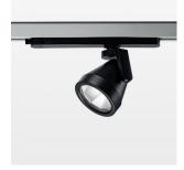
Surface-mounted luminaire with LED, rated life of the LED L80/B10 > 50000 h, colour rendering index CRI > 90, chromaticity tolerance 2 SDCM (initial), reflector with oval light distribution pattern, reflector pure aluminium 99,99% in MIRO-Silver®, rotation angle 330°, swivel angle +85°/-85°, luminaire head/retention arm die-cast aluminium, powder-coated, stratoblack
