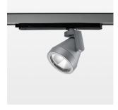
Surface-mounted luminaire with LED, rated life of the LED L80/B10 > 50000 h, colour rendering index CRI > 96, chromaticity tolerance 2 SDCM (initial), reflector with oval light distribution pattern, reflector pure aluminium 99,99% in MIRO-Silver®, rotation angle 330°, swivel angle +85°/-85°, luminaire head/retention arm die-cast aluminium, powder-coated, stratosilver
