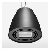
Suspended luminaire with LED, rated life of the LED L80/B10 > 50000 h, colour rendering index CRI > 80, chromaticity tolerance 3 SDCM (initial), reflector with double asymmetrical light distribution pattern, reflector pure aluminium 99,99% in MIRO-Silver®, luminaire housing sheet steel, powdercoated, stratoblack
