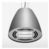
Suspended luminaire with LED, rated life of the LED L80/B10 > 50000 h, colour rendering index CRI > 80, chromaticity tolerance 3 SDCM (initial), reflector with double asymmetrical light distribution pattern, reflector pure aluminium 99,99% in MIRO-Silver®, luminaire housing sheet steel, powdercoated, stratosilver
