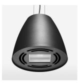
Suspended luminaire with LED, rated life of the LED L80/B10 > 50000 h, colour rendering index CRI > 80, chromaticity tolerance 3 SDCM (initial), reflector with double asymmetrical light distribution pattern, reflector pure aluminium 99,99% in MIRO-Silver®, luminaire housing sheet steel, powder-coated, stratoblack
